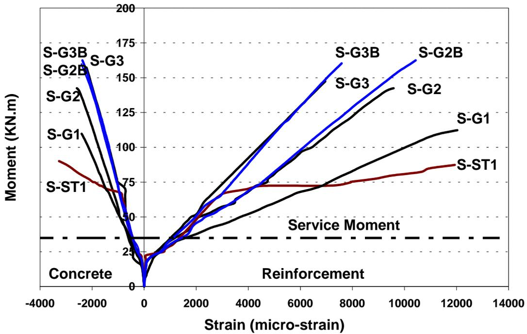
(b) Slabs reinforced with glass FRP bars and one control
