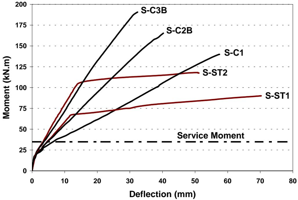
(a) Slabs reinforced with carbon FRP bars and the two controls
