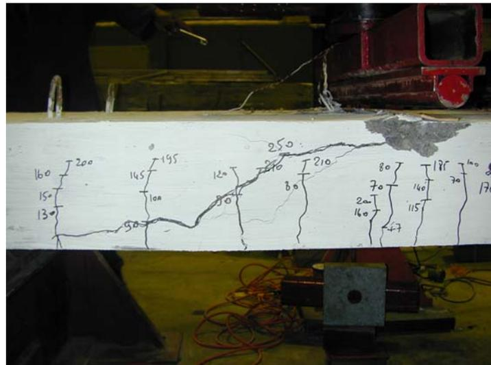
(b) Compression-shear failure (S-C2B)
