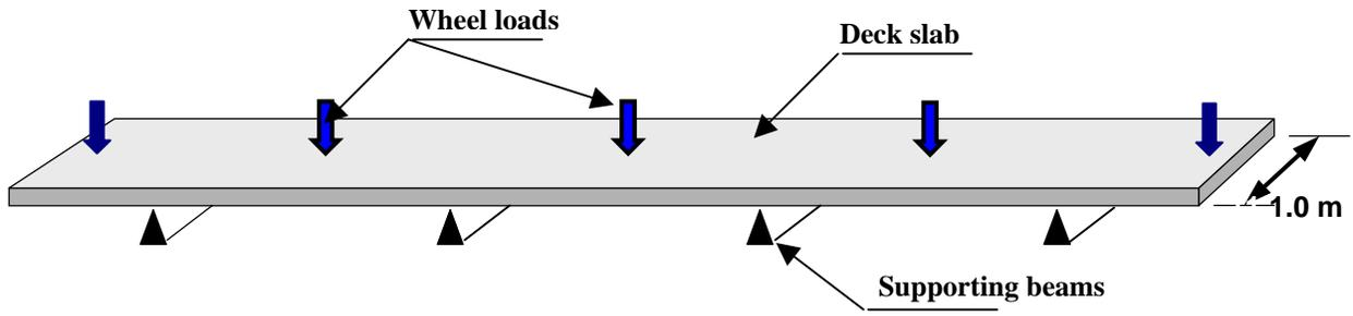
(a) Design strip of a bridge deck slab
