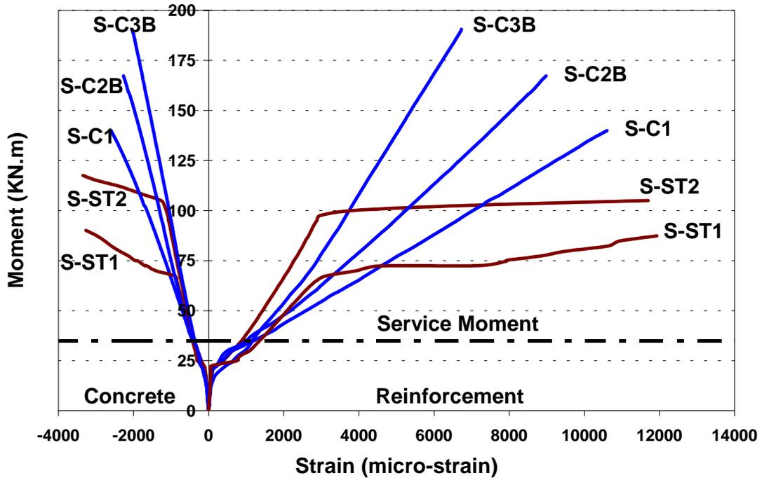
(a) Slabs reinforced with carbon FRP bars and the two controls
