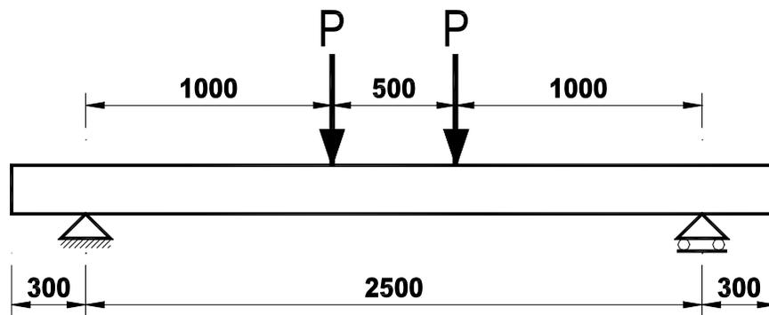
(b) Schematic drawing of the test set-up
