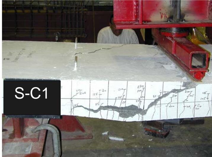
(a) Tension-shear failure (S-C1)
